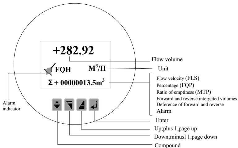
Note: When measuring, pushing down “Compound Key + Enter” will appear password of changing state, base on distinction of secrecy, and change the password as we provide. Then pushing “Compound Key + Enter” again, and you can inter the state of setting parameter. If want to return to the running state, push “Enter” for several seconds.
