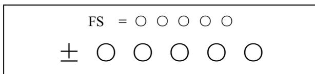
Converter's zero-flow correction displays like this:
