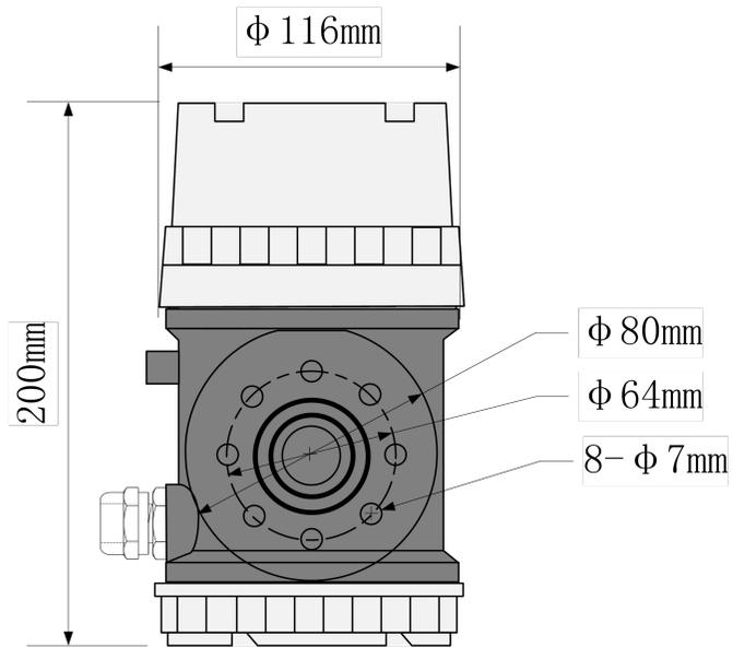
Fig.1.3 L-mag 511B series 511C Shell
