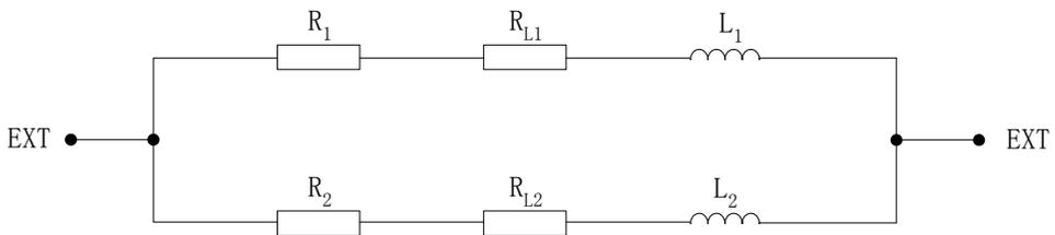
Total resist =  $(R1 + R_{L1})$  parallel connection  $(R2 + R_{L2}) \leq 120\Omega$ ;
