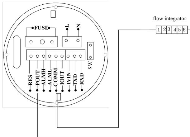
Figure 4.4.2 (c) Connection of Electronic Counter
