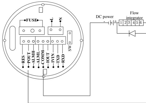
Fig 4.4.2(b) Connection of Electro-Mag 511Bnet Counter
