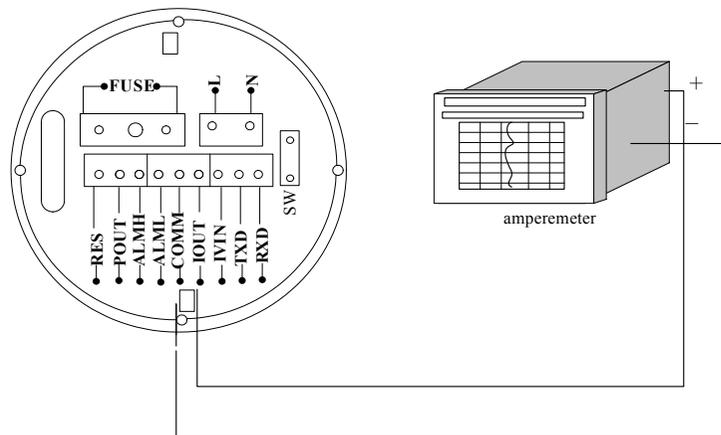
Fig.4.4.2(a) Output and power supply cables
